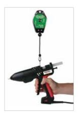
If the tool is being used for repetitive work over a work surface, then the tec SB-1200 spring balancer is an economic tool support system with easily adjustable tension control. Capable of supporting tools up to 1.5 kilos (3.3lbs) in weight, it has a maximum extended cord length of 1.6 metres (5ft).
