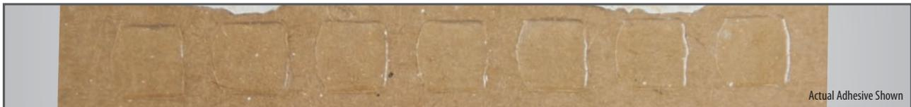
QDP Adhesive Pattern Sample 9mm x 10mm pattern spaced 14mm on center
