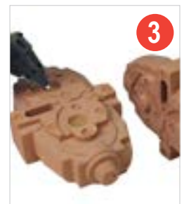
Assembly of sand cores for cylinder blocks
