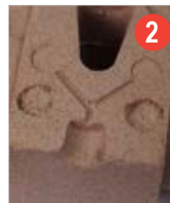
Sand cores showing recesses required for hot melt
