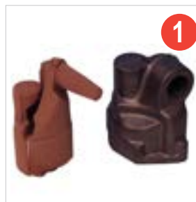
Internal sand core shape, and finished pump casting
